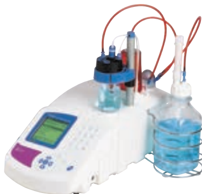
Basic Titrator—perfect for QC labs that always run the same samples
