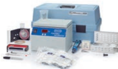
This economical portable lab monitors key water quality parameters plus Total Coliforms and E. coli using presence-absence method. Filtration and incubation consumables only. Order media separately.
